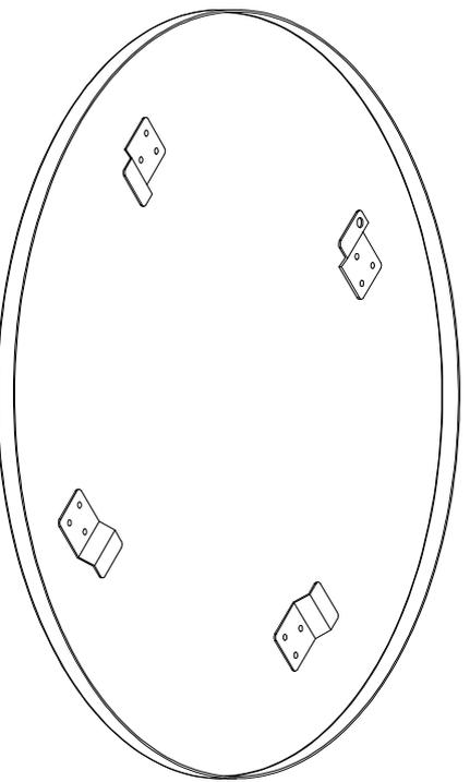
UNIONE TRAMITE ELETROPUNTATURA Ø6
